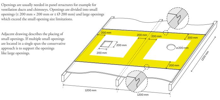
Figure 20. Placing of small openings
