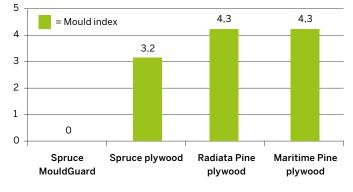
Figure 47. Results of the outdoor field test by VTT (VTT-R-10360-10), mould index describes the occurence of mould growth on the panel surface
