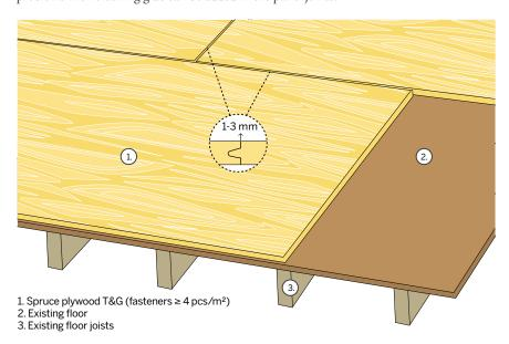
Figure 36. Spruce plywood installed directly on top of an existing floor
