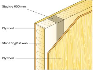
Figure 57. Example of a fire rated structure for a compartment wall
