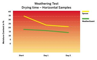
Flgure 49. Drying time of Spruce WeatherGuard and untreated spruce plywood measured by Metsä Wood.
