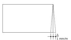
Figure 67. Straightness of a panel edge
