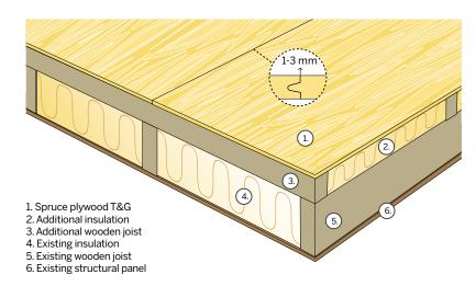
Figure 40. Additional insulation for base floor
