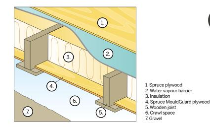
Figure 1. Typical ventilated wood floor structure
