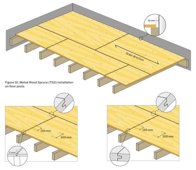
Figure 11. Metsä Wood Spruce (TG2) panel installation on floor joists
