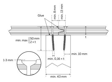
Figure 14. Fixing of TG panels to wooden support
