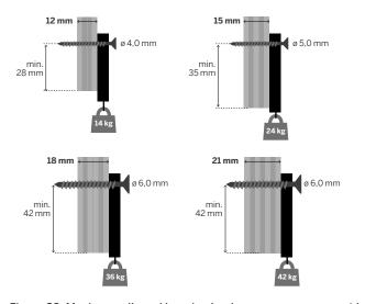
Figure 32. Maximum allowed hanging load per screw, permanent load duration class, service class 1 and 2, screw's characteristic tensile strength  $f_{u,k} \ge 500 \ N/mm^2$
