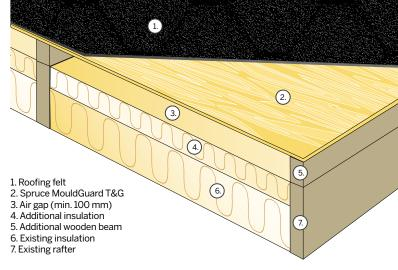
Figure 43. Additional insulation for roof
