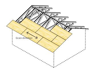
Figure 23. Panels are laid and fastened on wood trusses or rafters. The short edges of the panels are staggered.
