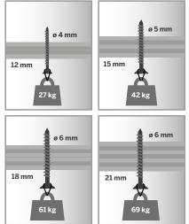
Figure 29. Maximum allowed hanging load per screw, permanent load duration class, service class 1 and 2
