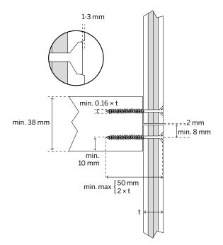
Figure 33. Fixing to wooden support by wood screws
