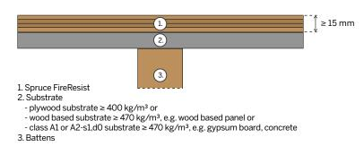
Figure 56. Floor structure with Spruce FireResist fixed to the substrate
