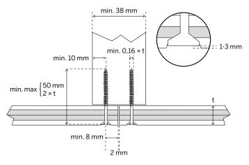
Figure 27. Fastening ceiling panels under the rafters/joists
