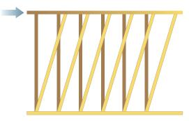
Figure 31. Laterally loaded wall structure without panel bracing
