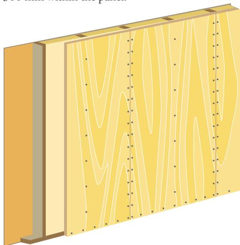
Figure 30. Panel bracing
