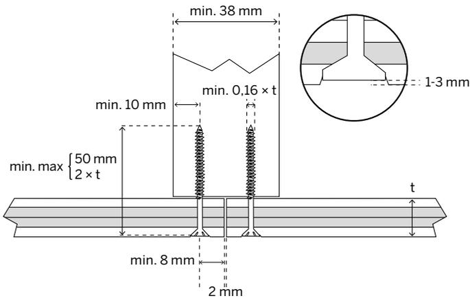
Figure 27. Fastening ceiling panels under the rafters/joists
