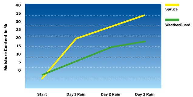
Figure 48. Water absorption of Spruce WeatherGuard and untreated spruce plywood measured by Metsä Wood.
