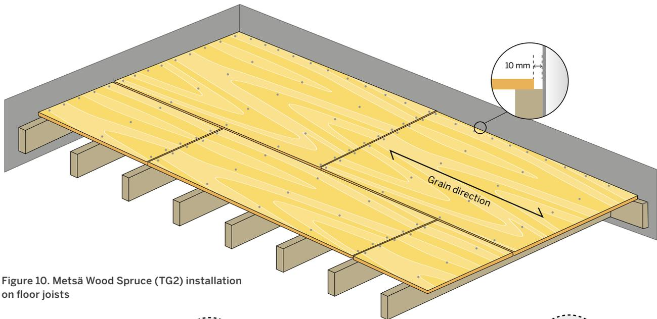
Figure 10. Metsä Wood Spruce (TG2) installation on floor joists
