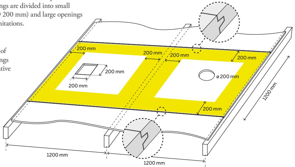
Figure 20. Placing of small openings
