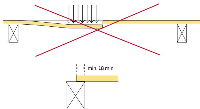
Figure 15. Unsupported square panel edges are not allowed, also short edges of tongue and grooved panels should be placed on supports
