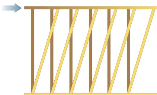
Figure 31. Laterally loaded wall structure without panel bracing
