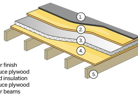
Figure 5. Floating floor (wood based)
