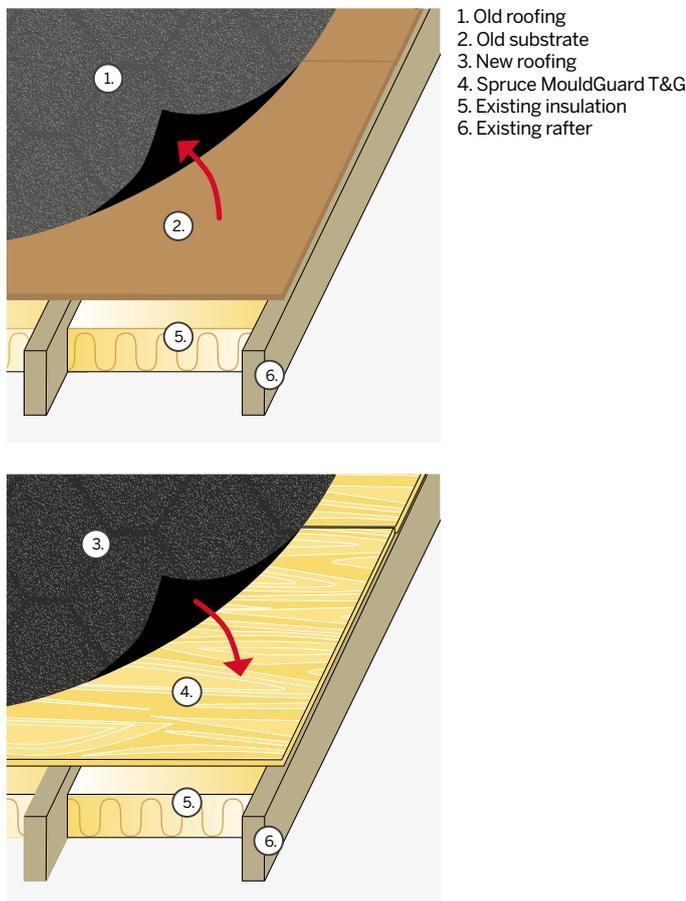
Figure 41. Replacing old surface structures of a roof
