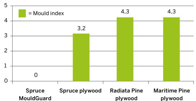
Figure 47. Results of the outdoor field test by VTT (VTT-R-10360-10), mould index describes the occurrence of mould growth on the panel surface
