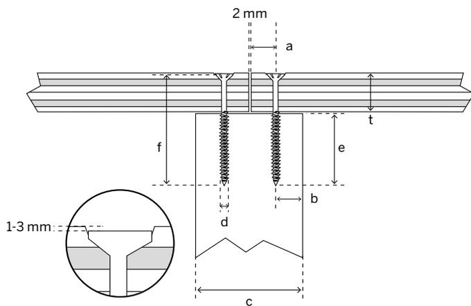
Figure 70. Fixing of square edge panels to wooden supports according to EN 1995-1-1
