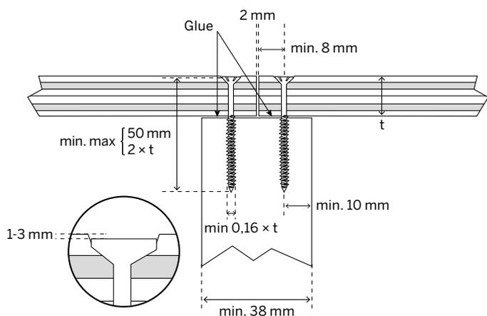
Figure 13. Fixing of square edge panels to wooden support
