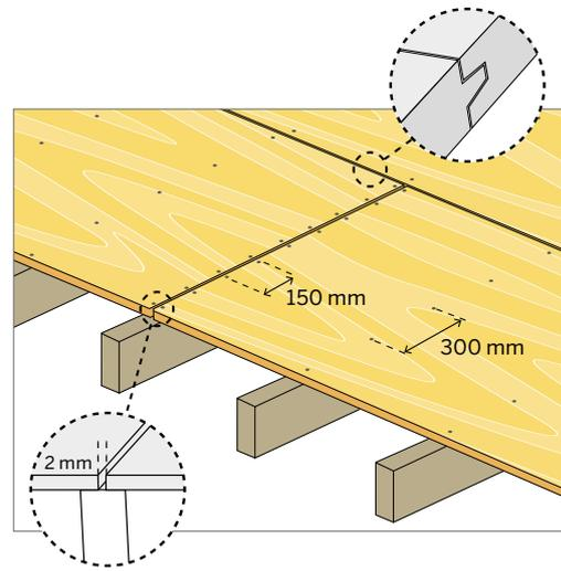
Figure 24. Metsä Wood Spruce (TG2) panel installation on rafters
