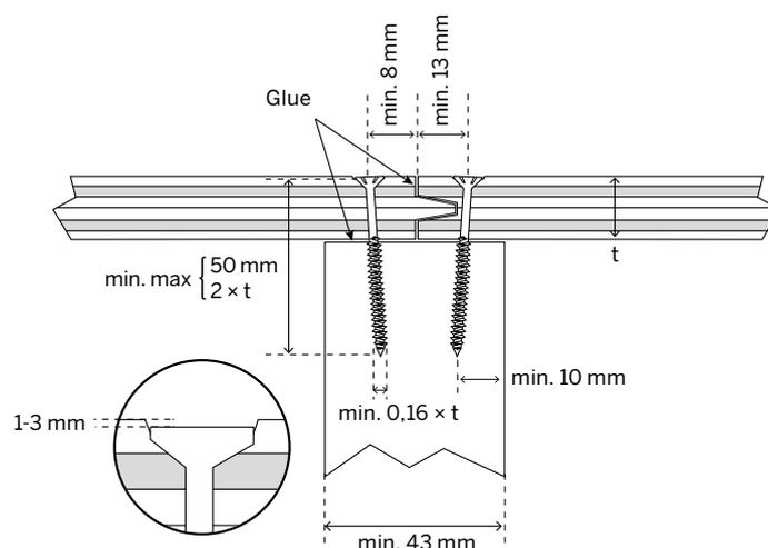
Figure 14. Fixing of TG panels to wooden support
