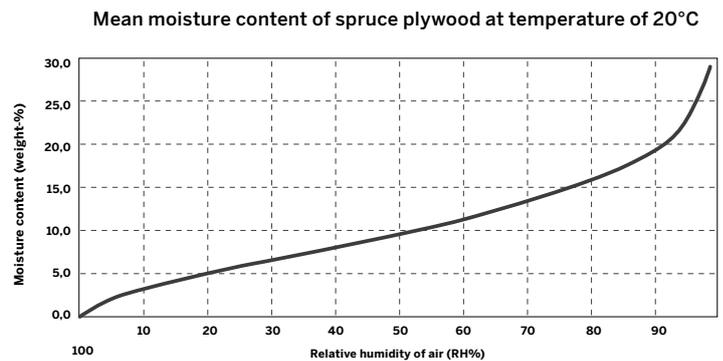
Figure 69. Mean equilibrium moisture content of spruce plywood
