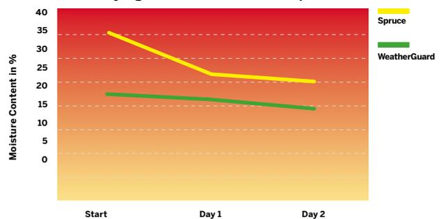
Figure 49. Drying time of Spruce WeatherGuard and untreated spruce plywood measured by Metsä Wood.
