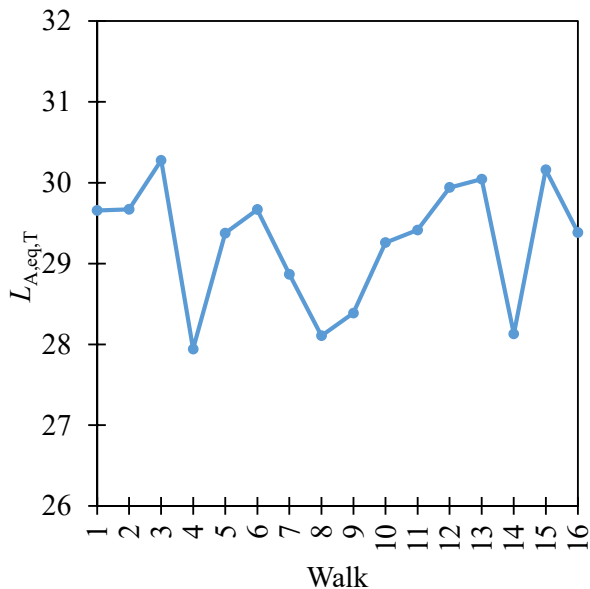
Fig. S6. Typical variation of the A-weighted SPL between successive walkthroughs. The example concerns floor type C2 .
