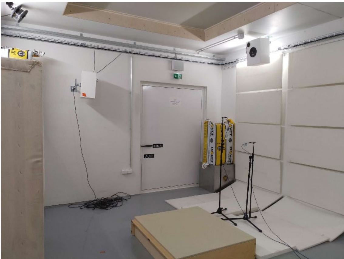
Fig. S10. Placement of the absorbers in the impact sound insulation laboratory during the recording of natural impact sounds. The loudspeaker shown in three figures was not present during the recordings. The positions of the recording microphones are also shown.
